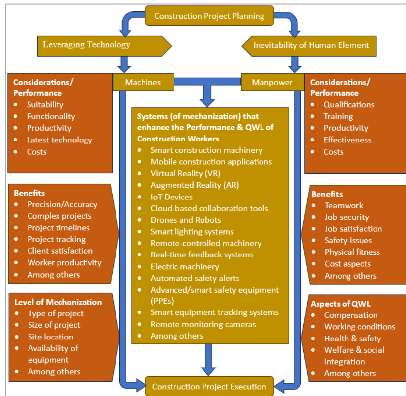
Figure 5: : Framework for Optimizing the Level of Mechanization and Manpower in Construction Projects in Kenya
